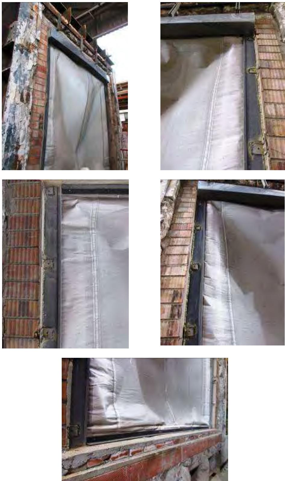
PHOTOS No.15,16,17,18,19: Details of the barrier once the test has ended at minute 181.
