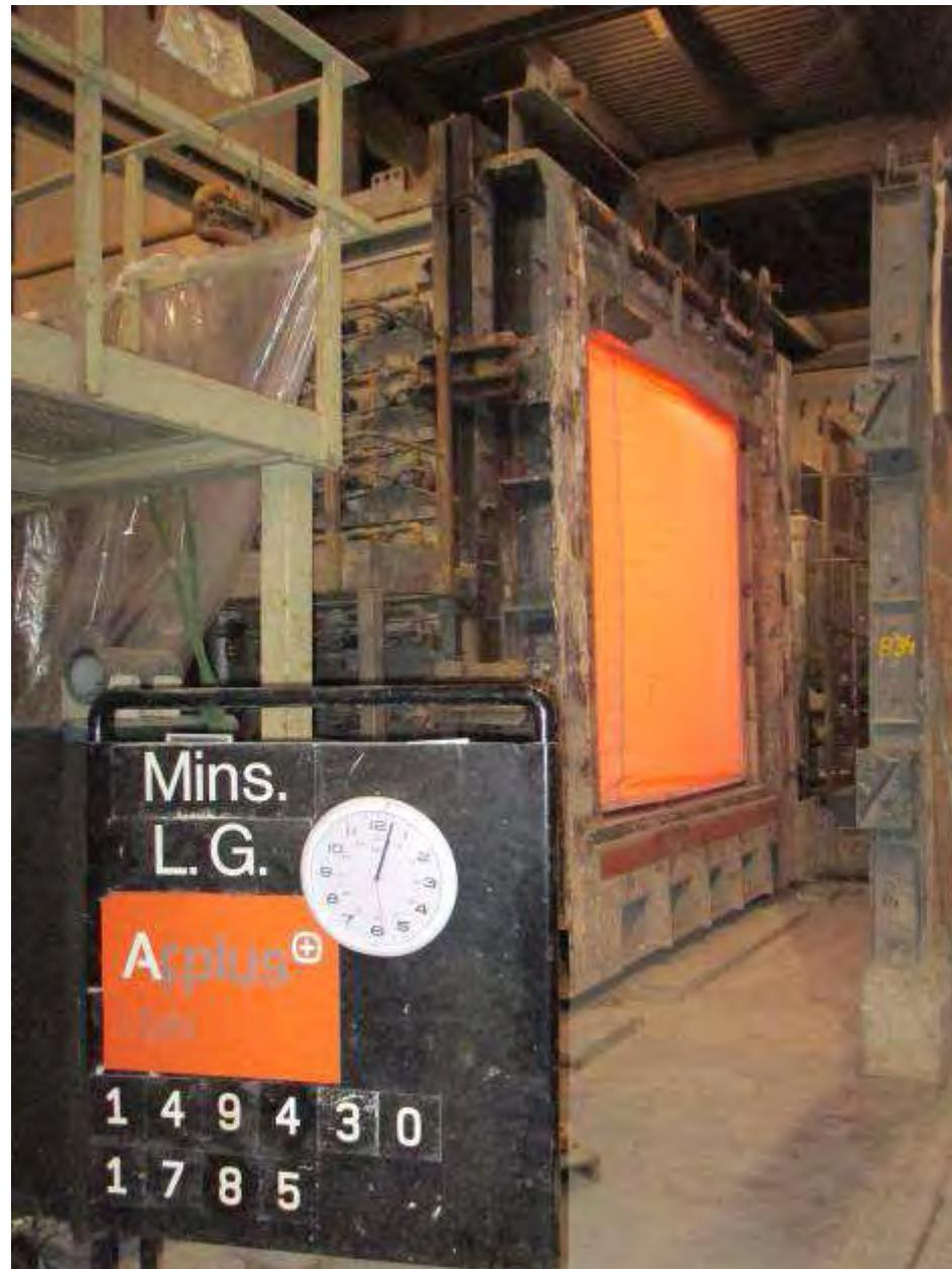
PHOTO No.10: General view of the sample and .the furnace at minute 60 of the test
